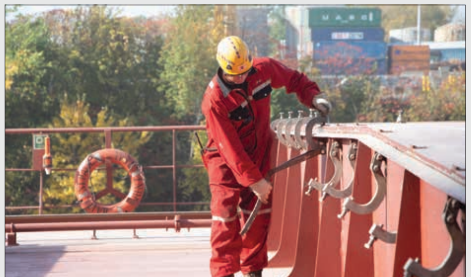
Securing Cargo Holds (CSL Baie St. Paul)
