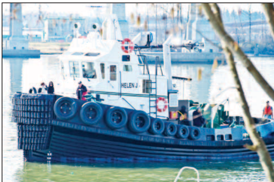
Jones Marine's new tug, the Helen J is 50 feet long, a beam of 21 feet and has power of 1700 hp. The Helen J brings Jones Marine fleet to ten vessels.
