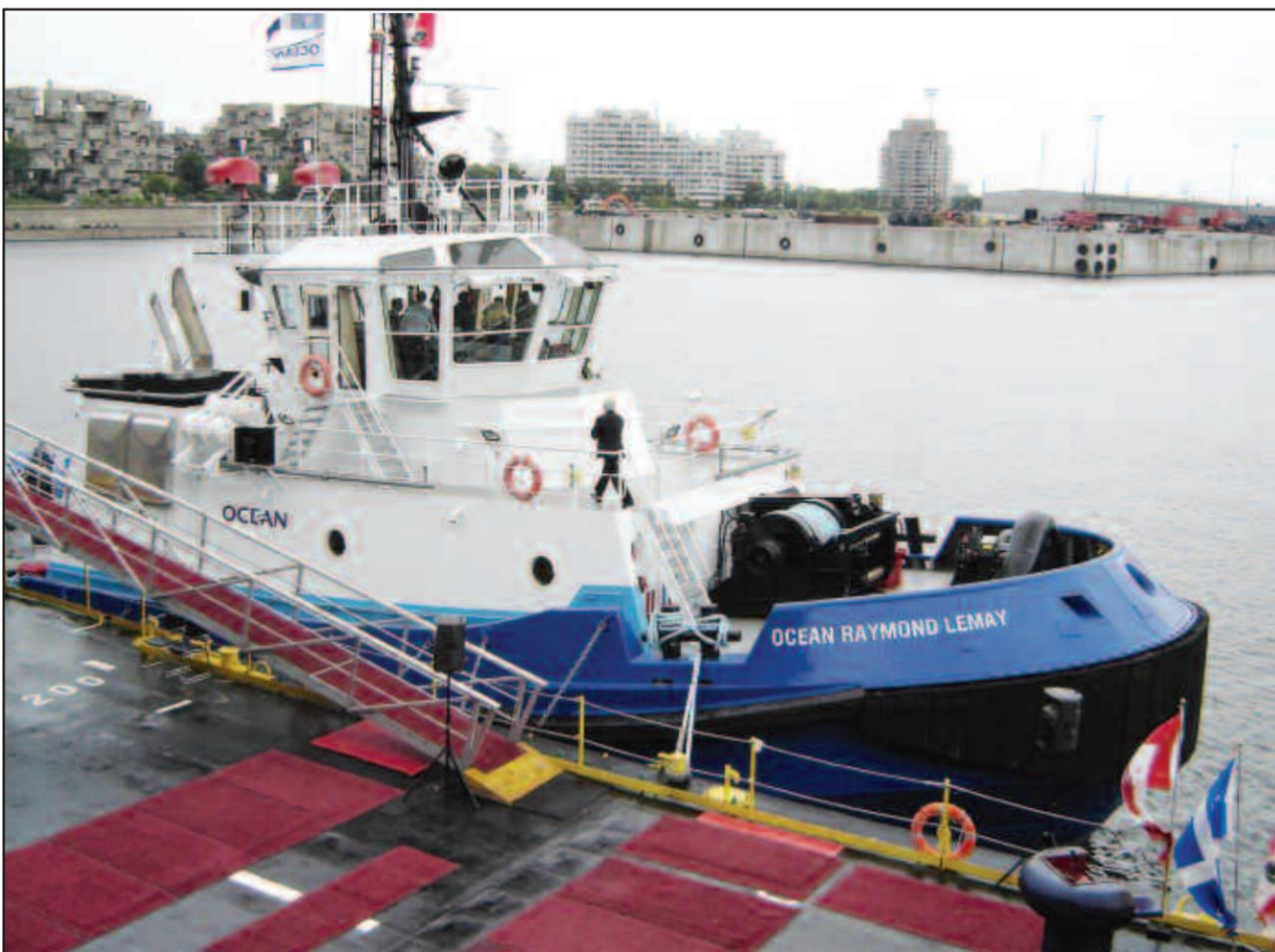
Groupe Océan has added a new vessel to its fleet. A state-of-the-art 5,000 BHP tugboat propelled by two Z-drive propellers, it features a Class 1 firefighting equipment and an Ice Class 1A hull.
