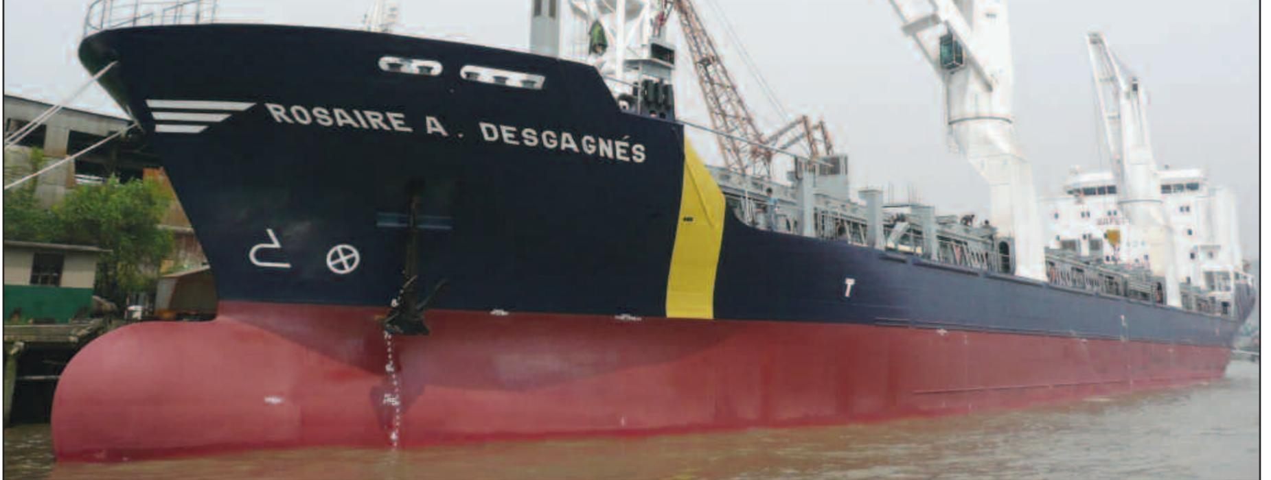
The Rosaire A. Desgagnés is the latest addition to Groupe Desgagnés' fleet. A tweendeck Lo-Lo (lift on-lift off) cargo vessel, it is equipped with two 120 mt cranes capable to lift 240 mt in tandem.
